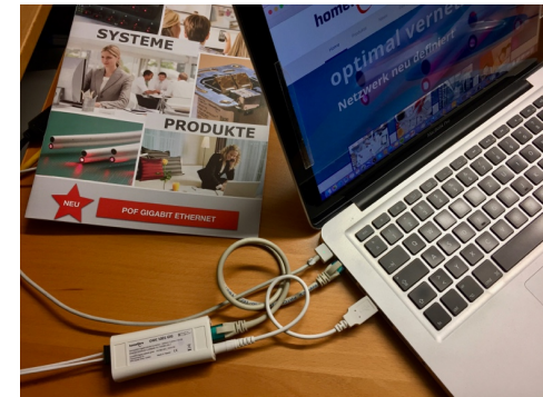
Gigabit Ethernet Interface 5V DC Power via USB or Power Supply
