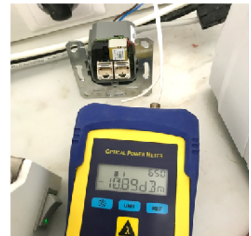
Check of signal strength with fresh cut POF-cable heads in 2022. About 10 years of operation did not affect the performance of the cable.
