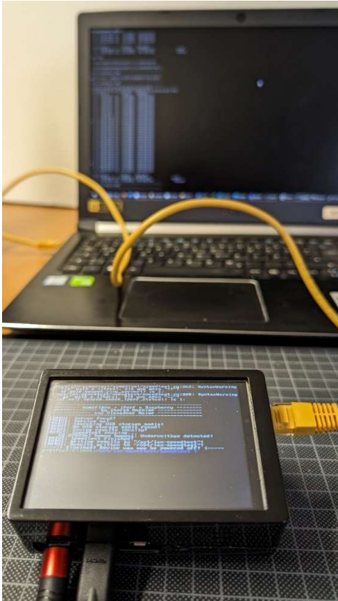
Fig. Raspberry IPERF Client and Notebook with IPERF Server.
